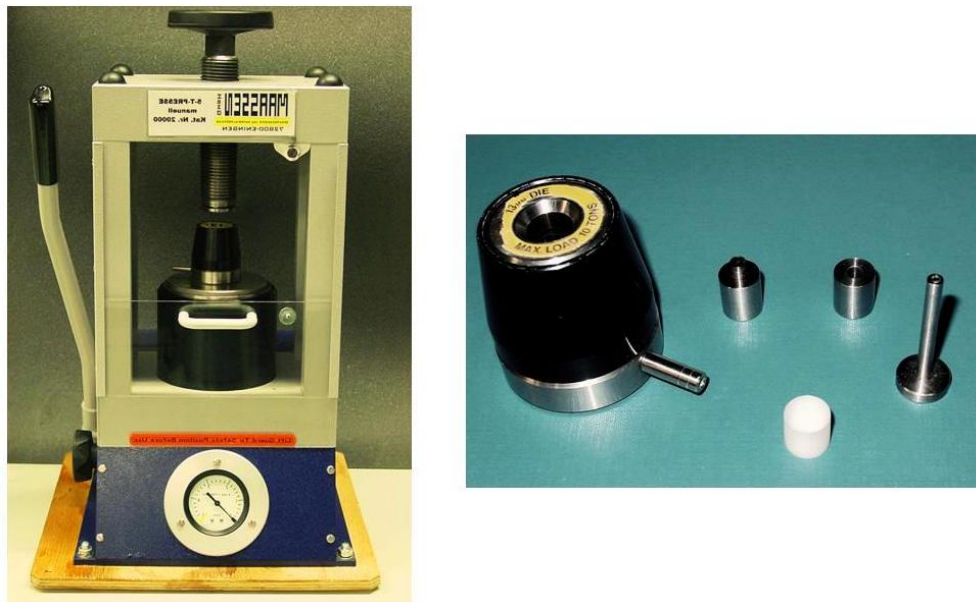
Figure 2.2.4 Hydraulic press and compacting equipment.
