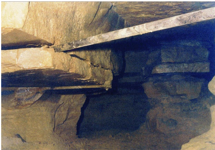
Figure 6 Material from the base of the limestone being removed from a mine for testing.
