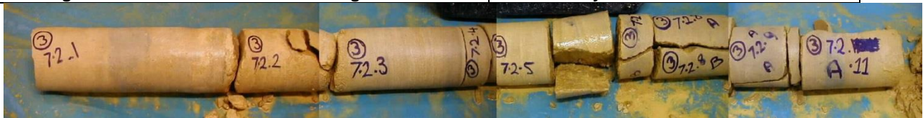
Figure 9 Composite photograph of a typical section of Collyweston Limestone borehole core
