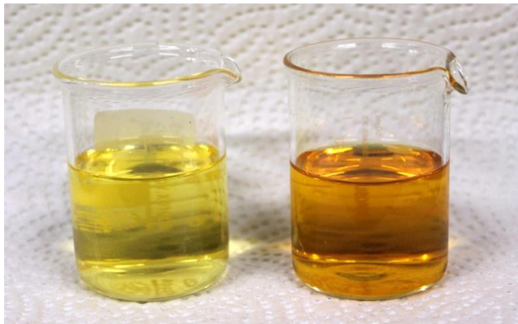
Figure 3.4: TiO 2 Precursor Solutions. a) TiO 2 standard precursor (left), b) TiO 2 precursor mixed with Urea (right).
