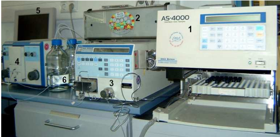
Figure 4 HPLC system for the measurement of TBARS plasma concentrations.
