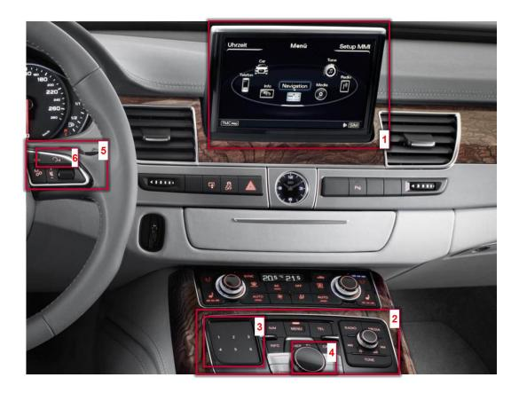
Figure 0.1.: Automotive infotainment system 1.GUI and central display 2.control unit 3.touch pad 4.turn-press button 5.multi-function-wheel 6.speech button
