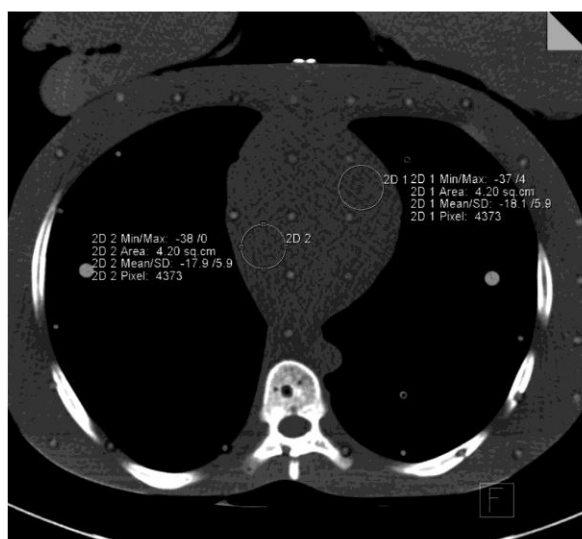
FIGURE 3. Example for density measurements. Two ROIs are placed in a homogeneous area of the phantom's mediastinum.
