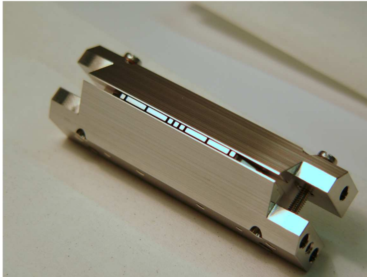
Figure 3.5.: One half of our linear endcap trap, we refer to Figure 3.3 for the electrode structure in radial direction. RF and DC signals are applied to different segments, while grounded endcap electrodes extend over the full length of the trap. For our spectroscopy (Chapter 4) and ion oscillator experiments (Chapter 5) we used a single long segment of the trap.
