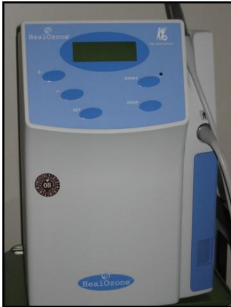
Fig. 1: The gaseous ozone generating device for oral application.
