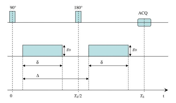
Figure 3.1: The sequence timing diagram illustrates the diffusion pulse sequence introduced by Stejskal and Tanner: its characteristic features are two strong symmetric gradient lobes placed on either side of the 180° refocusing pulse in a spin-echo sequence.  $\delta$  is the gradient duration and  $\Delta$ is the interval time between the onsets of the pulses.
