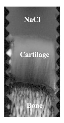
Figure 4.4: For MRI measurements, the samples were put in a hollow Plexiglas cylinder (free inner diameter = 7 mm, outer diameter = 10 mm) filled with physiological saline. The diffusion measurement with b = 0 gives a  $T_2$ weighted image: saline solution (NaCl), cartilage and bone were well distinguishable.
