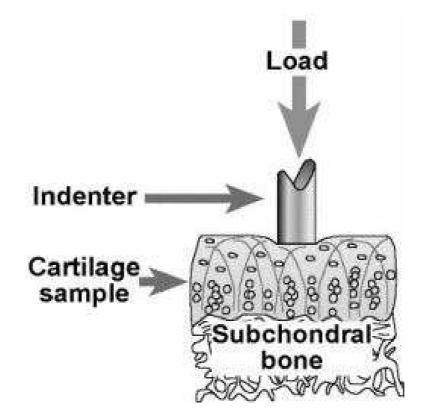
Figure 6.2: The indentation experiment simulates better than other mechanical tests the anatomical loading on the cartilage in the body: the load is local, the cartilage is still anchored to the bone and the cartilage fluid can move freely in the sample.
