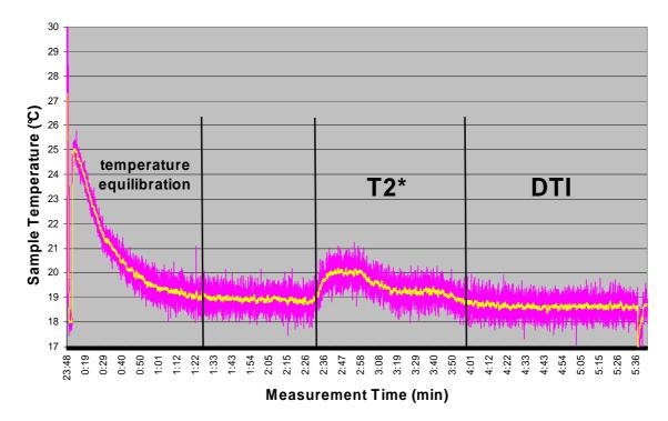
Figure 5.5: The temperature of the sample was measured during the entire experiment. About 1 hour after the start, the sample had the same temperature as the gradient system. Standard diffusion-weighted sequences do not cause a significant increase in the temperature. Pink are the experimental values and yellow the averaged values.
