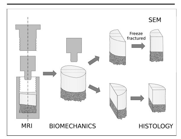
Figure 6.1: Schema of the experiment design. First, MRI was performed with and without mechanical loading. Second, the sample was tested for biomechanics: the load was applied from the indenter on the region of the MRI slice. Than the sample was cut perpendicular to the MRI slice and further analyzed in SEM and histology.
