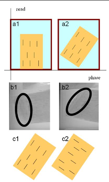
Figure 5.8: The anisotropy of the phantom is known. a) Schematic representation of the anisotropic phantom in two different positions: a1) main anisotropy parallel to the read direction; a2) main anisotropy in the diagonal between read and phase direction; b) Our phantom was a part (encircled) of a carrot with known fiber structure; c) After the measurement, the data were processed.
