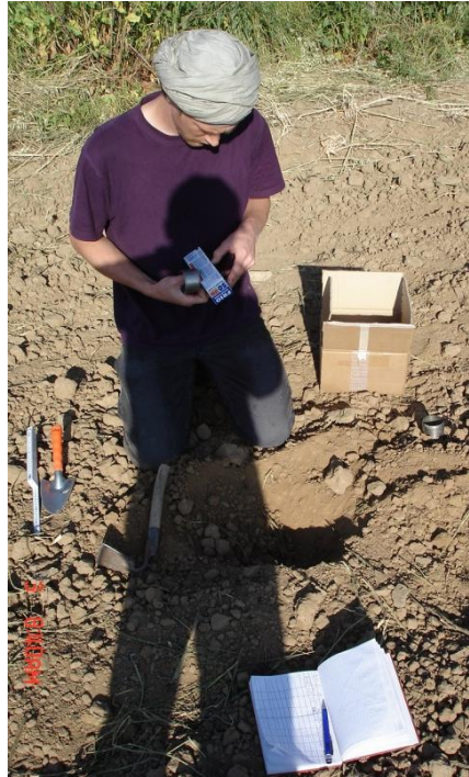
Figure 3.8 Taking soil samples for gravimetric soil moisture. In the photo: Seppo Schmid and the shadow of the author. Date: 3 rd May 2008.
