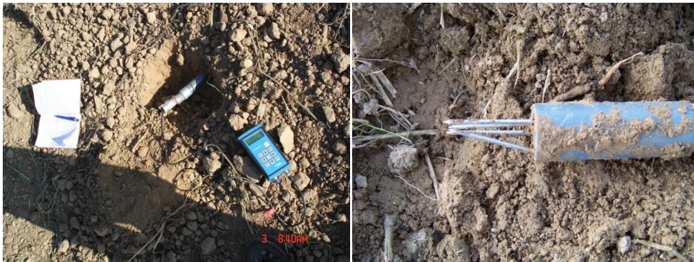
Figure 3.10 UMS INFIELD7 (left) and a broken ThetaProbe ML2x probe (right).
