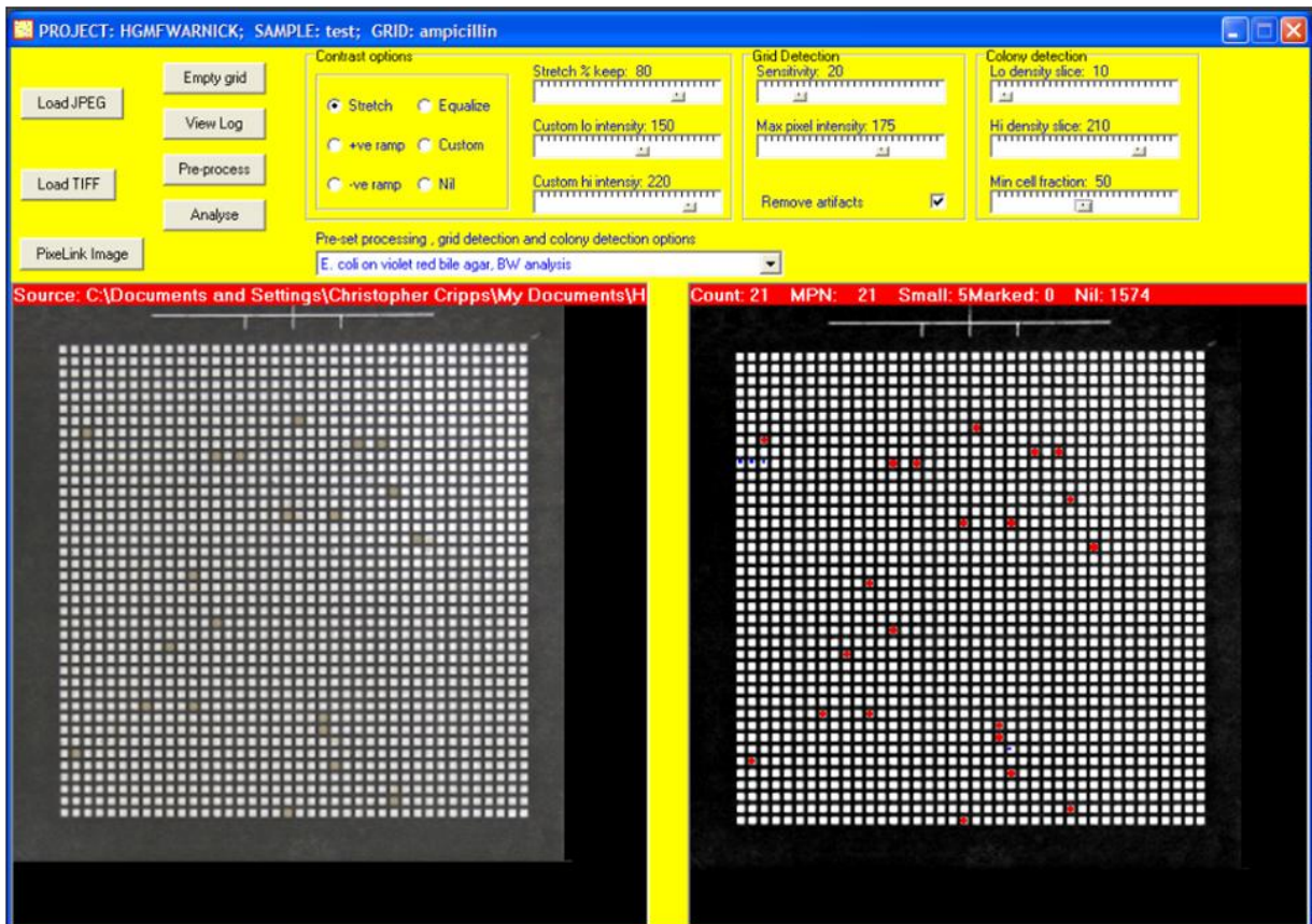
Figure: HGMFRES software, NSW Department of Primary Industries, Wollongbar, NSW, Australia. Original digital picture of the grid to be analyzed on (left), analyzed grid with colonies being highlighted in red (right).
