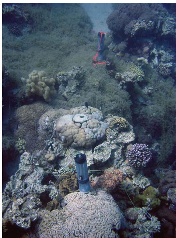
Fig. 1 In situ O_2 loggers deployed at adjacent reef sites dominated by scleractinian corals or benthic macroalgae
