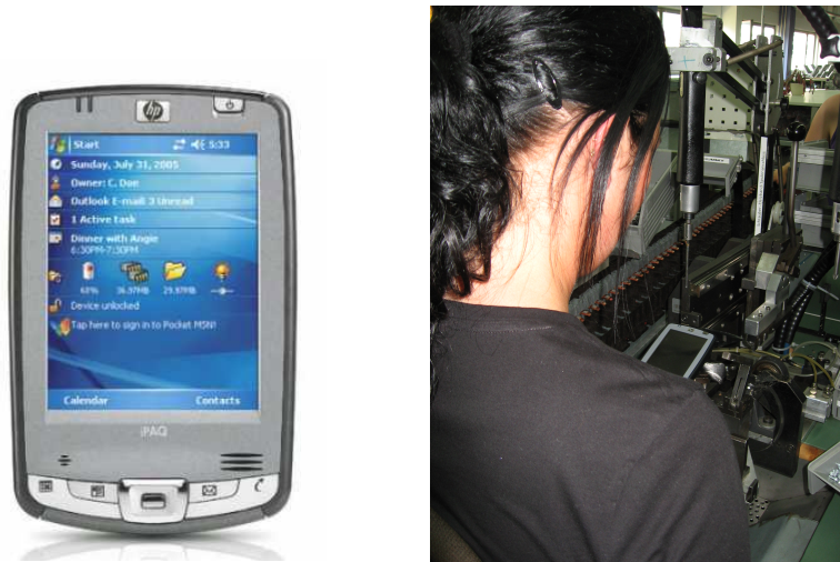
FIGURE 3.4. The HP iPAQ pocket PC (sketched on the left side) was ideally suited for the field experiments (see right side for a Pocket PC in use during the field study). It disposed of a relatively large screen and the two outer buttons could be used as response buttons.
