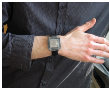
FIGURE 2.5. The Daqtometer - continuous recordings of both, changes in dynamic and static acceleration (i.e. motion and gravity) allow for an appreciation of loco-motor activity for up to six months.
