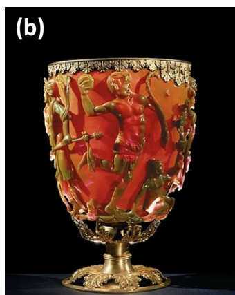
Figure 2.1 | The Lycurgus Cup is an excellent example of the optical properties of gold. (a) When illuminated from the outside, the gold nanoparticles inside the glass cup scatter the light, making the cup appear green. (b) However, when a light is placed inside the cup, the absorption of the gold nanoparticles changes the cup's apparent color to red.
