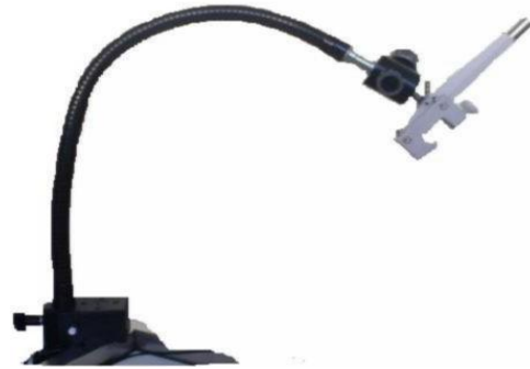
Figure C.6: Definitive holding Device for the Cytoscan® imaging probe.
