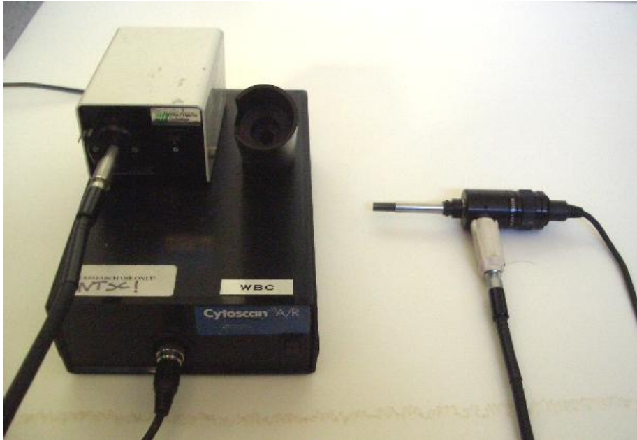
Figure C.3: Parts of the device: Probe (right), light source (metallic box) and CCD camera (black box).
