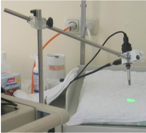
Figure C.5: First holding Device for the Cytoscan® imaging probe.
