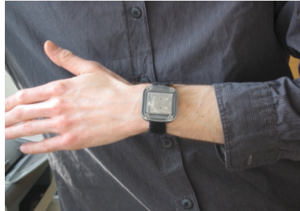
Figure 2.1. The Daqtometer ® is a wrist worn device to measure activity.
