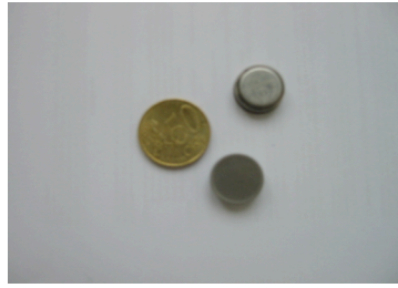
Figure 2.2. iButtons ® are small chips, the size of a wrist watch battery to assess distal and proximal body temperature
