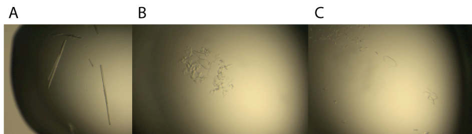
Figure 2-18. Crystals of D. melanogaster Pur- \alpha repeat III. A: Pur- \alpha 188-258 was crystallized at 4 °C A: Crystallization solution contained 100 mM sodium cacodylate pH 7.5, 0.2 M ammonium acetate, 15 % PEG 3350, and 4 % MPD. B: Crystallization solution contained 100 mM sodium cacodylate pH 7.5, 0.2 M sodium acetate, and 26 % PEG 3350. C: Crystallization solution contained 100 mM sodium cacodylate pH 7.5, 200 M sodium acetate, 22 % PEG 3350.
