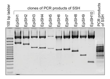
Suppl. Fig. 1. Fragments cloned from the PCR products of the suppression subtractive hybridisation. The ten different size classes are depicted. The vector is visible as a 3.9 kb band at the top of the ten lanes. PCR products are shown on the right for comparison. A negative image of an ethidium bromide-stained gel is shown. The size of the inserts surpasses that of the respective PCR products due to the presence of short vector fragments at both ends.
