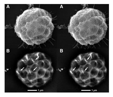
Suppl. Fig. 1. Stereo pairs of scanning electron micrographs of a MMP operated at 30 keV A. Filamentous surface structures observed in the secondary electron image. B. Back scattered electron image reveals the arrangement of single cells within an individual MMP. The rows of magnetosomes can be distinguished based on their high yield of backscattered electrons resulting in a bright signal.
