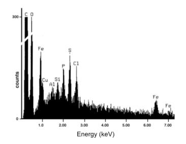
**Fig. 3.** Energy dispersive X-ray (EDX) analysis of an individual bullet-shaped magnetosome crystal. The prominent iron and sulfur peaks indicate the presence of an iron-sulfur mineral. Carbon, oxygen, aluminium, silicium, phosphor and chloride signals in the spectrum originate from the cellular background and the copper peak from the electron microscopy grid.
