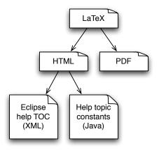
Figure 18.2: Help content. All of the help content is authored as LaTeX. From the LaTeX sources, HTML files and a PDF file a produced via standard tools. A custom process translates the HTML file to an Eclipse Table of Contents file and a Java source file with constants for context-sensitive help.
