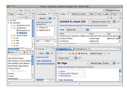
Figure 1.2: HYENA/Eclipse. The left column gives access to the projects and their files and gives access to common RDF management operations. Top center and right are "master" views for listing RDF resources. Bottom center and right are "detail" views for editing individual resources.
