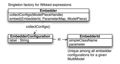
Figure 19.2: An embedder produces Wikked expressions and declares what it can embed by returning configurations.
