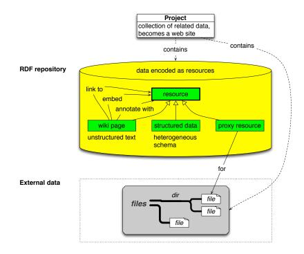
Figure 9.1: A project contains an RDF repository for managing all of the data and some external data that does not fit into the repository, but is instead represented by proxy resources.
