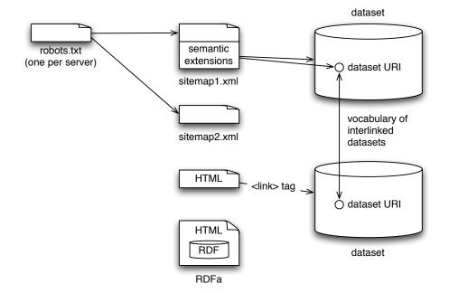
Figure 3.1: Datasets can be discovered by following the per-server robots.txt to semantic sitemaps. HTML files can refer to related RDF datasets, if those are stored in files. The RDFa standard allows one to embed related RDF data inside HTML. The RDF vocabulary of interlinked datasets is used to provide further meta data.
