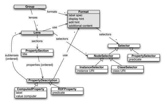
Figure 15.1: The main REMM presentation constructs are the group, the lens, and the format. A group contains lenses and formats. A lens contains properties partitioned into sections. Both formats and lenses use selectors to declare their applicability, but only the former can apply to properties.
