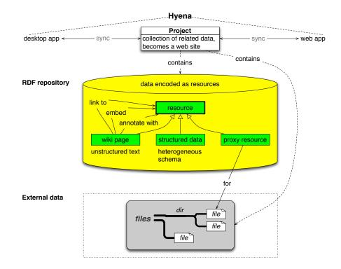
Figure 1.1: There are two versions of HYENA, a desktop version and a web application. Data is managed in *projects* and synchronized between the two. The dominant construct of a project is an RDF repository which is used to manage all of the data. Data that does not fit into the repository is kept externally and considered unstructured to HYENA. Currently only files are handled this way.
