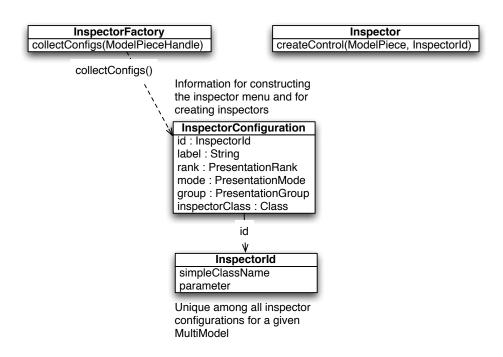
Figure 19.3: An inspector factory declares what can be graphically represented by returning configurations. An inspector is created from the class included in a configuration and initialized with a model piece and an ID.
