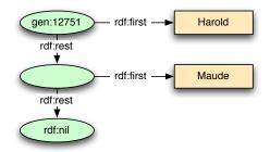
Figure 2.3: A collection with the member literals "Harold" and "Maude". The nodes on the right are those member literals. The nodes on the left are the data structure, a chain of resources connected via rdf:rest properties. The whole data structure has the URI gen:12751.
