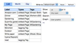
Figure 29.2: Master view, "List" tab. Displays resources in a table, each row holds a resource's label, its types and its tags. The table can be filtered via the controls to the right: One can limit the amount of resources displayed, one can filter by type, by text, or by graph (which are URI-named partitions of an RDF repository).
