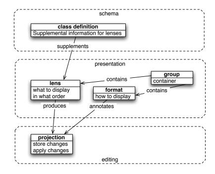
Figure 13.1: The REMM is partitioned into three layers: schema, presentation and editing. Except for projection (which is purely a programming language data structure) each of the constructs in the layers is defined by an RDF resource.
