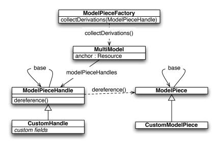
Figure 19.1: Model piece handles are produced by a factory and added to a multimodel. Each model piece handle points to at most one model piece handle it is derived from (its *base*). Model pieces also point to their base.
