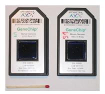
Figure 2.2: Two Affymetrix Microarray GeneChips<sup>®</sup> for Human (HG-U133 Plus 2.0) and Mouse Genome (Mouse-430 2.0).
