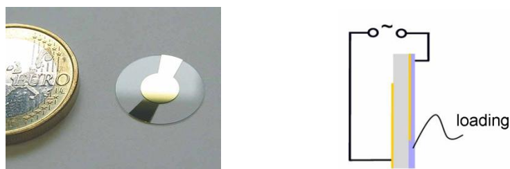
Fig. 17: 10 MHz quartz crystal microbalance
