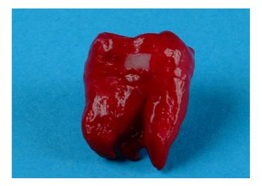
Fig. 7. Sample tooth painted with nail varnish, leaving an exposed window of enamel.
