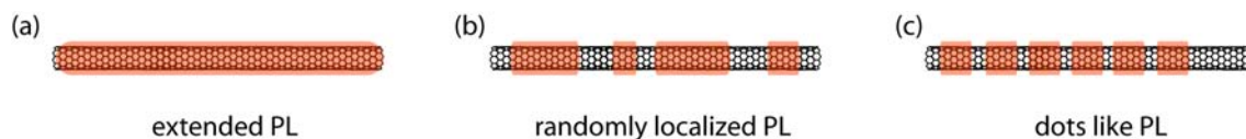
Figure 32: Illustration of PL along the nanotube with different extension. (a) Extended PL along the nanotube. (b) Localized PL along the nanotube. (c) Localized PL with regular spacing along the nanotube.
