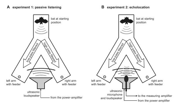
Figure 2.2: Y-shaped training platform. The bats were trained to wait at the starting position at the top of the the platform and to crawl to the end of one of the two arms after the presentation of a foreground signal. When the foreground signal was lowpass-filtered, they had to crawl into the left arm. When it was high-pass-filtered, they had to crawl into the right arm.
