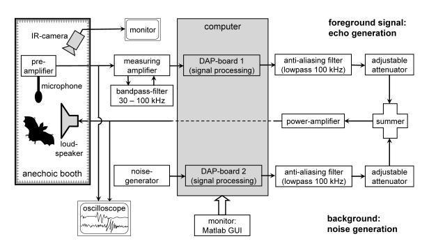
Figure 2.5: Block diagram of the stimulus generation- and presentation-setup in Experiment 2 (echolocation).
