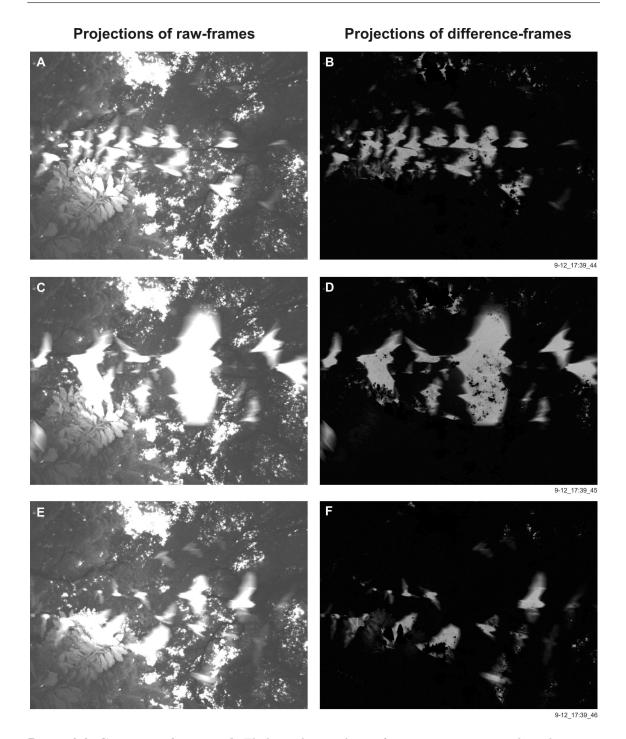
Figure 4.4: Camera-only control: Flight path recordings of two consecutive seconds without any object, except for the camera and infrared lightings on the ground. Every presented picture is the maximum-intensity-projection of 20 video-frames (667 ms recording time) onto one picture. Left column: The originally recorded 20 video-frames were directly used for the projection. Right column: The difference-frames between consecutive video-frames were calculated and then projected onto one picture.
