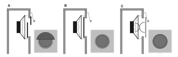
**Figure 3.5:** Sketch of the setup used to control for the perception of passive acoustic cues and air draught. The opening in front of the speakers was closed with different sets of disks to prevent the use of echolocation cues. The inset to the right of each sketch shows a frontal view of the occluded speaker.
