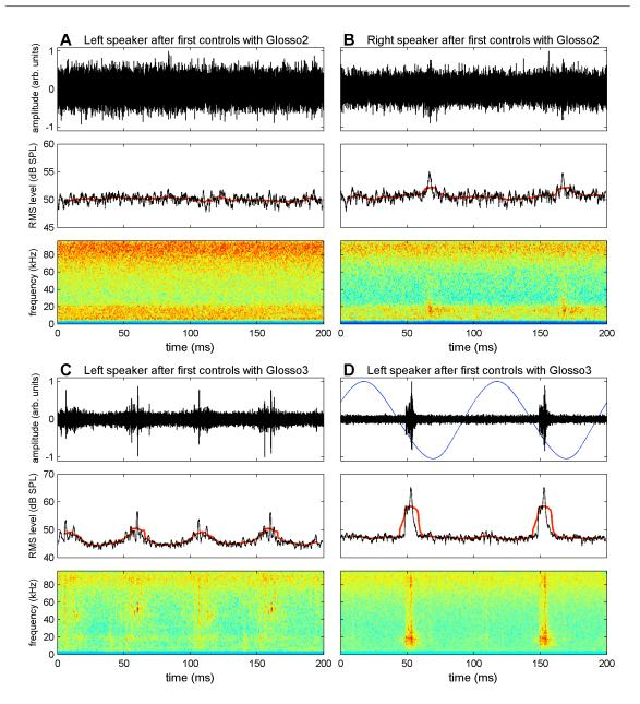
Figure 3.10: Sound recordings of the vibrating membranes, highpass filtered at 5 kHz and shown as time signal, running RMS-level (black: 1 ms integration window, red: 10 ms integration window) and spectrogram (512 point FFT, 97.5% overlap; the increase in energy above 80 kHz is caused by the microphone characteristics).
