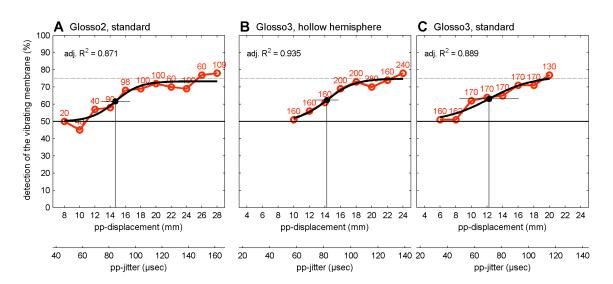
**Figure 3.7: Temporal jitter detection:** Temporal jitter detection performance (red) and the fitted psychometric functions (black) for a vibrating speaker membrane with 10 Hz vibration frequency for Glosso2 and Glosso3, using echo-acoustic cues. Note that the data were collected in the standard configuration with Glosso2 and in the hollow hemisphere and standard configuration with Glosso3.
