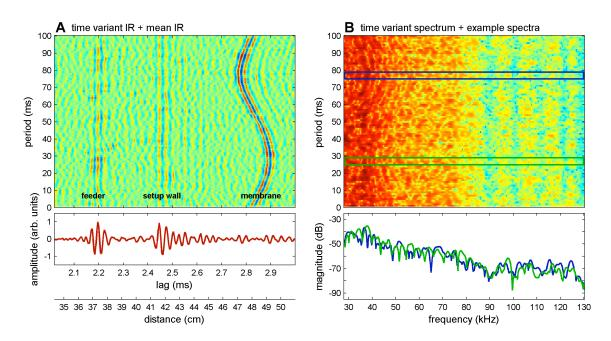
Figure 3.4: Time variant impulse response of the vibrating speaker membrane and its spectrum at a vibration frequency of 10 Hz with a pp-displacement of 22 mm (127  $\mu$ s time jitter). The vibrating membrane was ensonified with white noise and the reflected noise was recorded (sampling rate 260 kHz). A running cross-correlation between outgoing and reflected noise was calculated to extract the impulse response in steps of 1 ms of one vibration cycle.
