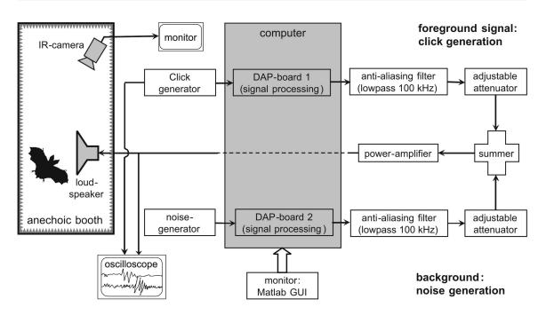
Figure 2.4: Block diagram of the stimulus generation- and presentation-setup in Experiment 1 (passive hearing).
