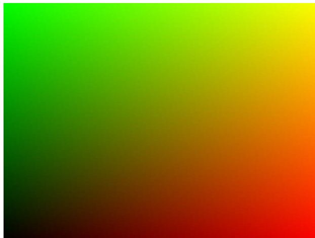
Figure 4.9: A two-dimensional colour space formed by additive colour mixture of red and green.
