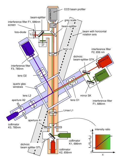
Figure 2.6: The principe of 3D measurements. The distribution of particles in volume is illuminated by the beam with perpendicular gradient of color. The x and y coordinates of particles are obtained from the xy projection, the z coordinate is determined from the ratio of color distribution. The picture is taken from [95].
