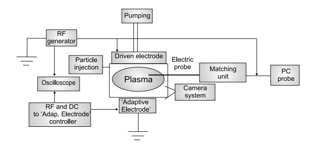
Figure 2.1: The sketch of the set-up with metallic wall chamber.
