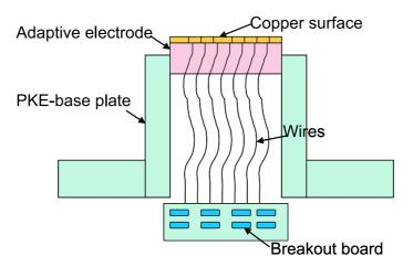
Figure 2.8: The sketch of the "adaptive electrode" mounting.
