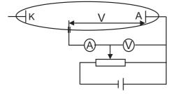
works during the years 1923 to 1935 [21]. Essentially, the electric probe is a small metallic electrode (usually, a wire), which is immersed into a plasma. The probe is connected to a power supply, which allows to maintain the different voltages on the probe (positive or negative with respect to the plasma potential). From the current gathered by the probe the different plasma parameters can be extracted. The simplest circuit of the probe measurements is shown in Fig. 1.1.
