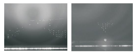
Figure 2.11: The possible configurations of the pixel connections. The switch open gives particles repulsion (left picture), while the switch closed gives particles attraction (right picture). In this case particles can be re-injected in plasma. 1-is the grounded surface of the chamber, 2-connected pixel, 3-RF voltage to pixel, 4-capacity, 5-inductance and 6-switch (left).
