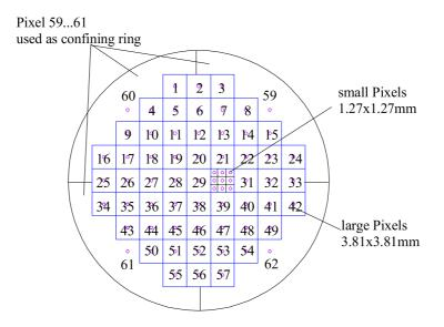
Figure 2.7: The "adaptive electrode" configuration seen from top.
