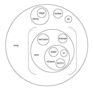
Figure 3.2: Base type system hierarchy
