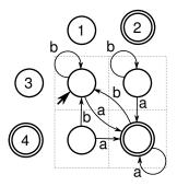
Figure 6.2: The product automaton on the right accepts the intersection of the language of the two automata on the left.
