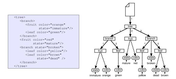
Figure 2.2: This example extends the apple tree example in figure 2.1 such that the elements are annotated using attributes. Elements may contain arbitrarily many attributes, but not two may have the same name. Note, that attributes have no explicit order in which they occur.
