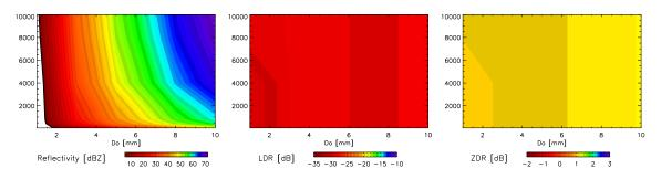
Figure 4.2: Reflectivity [dBZ],  $L_{DR}$  [dB], and  $Z_{DR}$  [dB] as a function of mean diameter  $D_o$  [mm] and intercept parameter  $N_o$  [mm<sup>-1</sup> m<sup>-3</sup>] for dry ice particles with a fixed density of 0.3 g cm<sup>-3</sup>, an axis ratio of 0.4, and a maximum canting angle of 40°.
