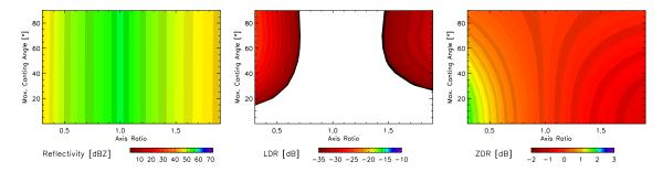
Figure 4.3: Reflectivity [dBZ],  $L_{DR}$  [dB], and  $Z_{DR}$  [dB] as a function of axis ratio and maximum canting angle for dry particles with  $N_o = 4000 \text{ mm}^{-1} \text{ m}^{-3}$ ,  $D_o = 5 \text{ mm}$ , and density  $\rho = 0.3 \text{ g cm}^{-3}$ .
