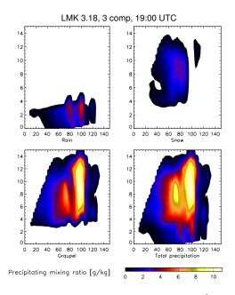
**Figure 4.9:** Vertical cross section of precipitation mixing ratios  $[g kg^{-1}]$  for the single hydrometeor types and total precipitation at 19:00 UTC on August 12th, 2004 (LMK 3.18, 3 component scheme).
