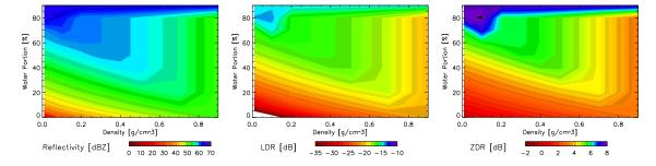
Figure 4.4: Reflectivity [dBZ],  $L_{DR}$  [dB], and  $Z_{DR}$  [dB] as a function of density [g cm<sup>-3</sup>] and water portion [%] in melting ice for  $N_o = 800 \text{ mm}^{-1} \text{ m}^{-3}$ ,  $D_o = 5 \text{ mm}$ ,  $\vartheta = 40^{\circ}$ , and  $\alpha = 0.3$ .
