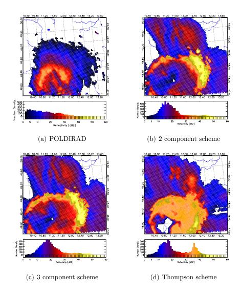
Figure 5.3: Observed and simulated 1° PPI scans of reflectivity [dBZ] at 8:00 UTC for July 5th, 2005 derived from simulations of the LMK 3.17 considering the 2 component, the 3 component, and the Thompson scheme. Below the figures, the legend gives colour coded reflectivity levels in dBZ as well as the number of pixels within the given reflectivity interval as a histogram.
