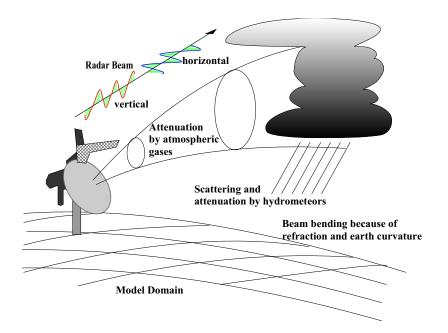
Figure 3.1: Conceptual view of the physical processes represented by the polarimetric radar forward operator SynPolRad (Synthetic Polarimetric Radar).
