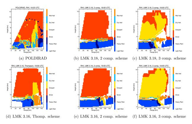
Figure 6.16: Hydrometeor classification derived from observed (19:23 UTC) and simulated polarimetric quantities for different model versions of the LMK at 19:00 UTC.
