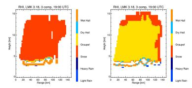
Figure 4.13: Hydrometeor classifications derived from the synthetic polarimetric quantities for the SynPolRad simulations only considering snow (left) and graupel (right).
