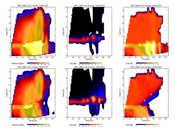
Figure 4.15: Synthetic RHI of reflectivity [dBZ],  $L_{DR}$  [dB], and  $Z_{DR}$  [dB] considering all precipitating hydrometeors in the upper row without and in the lower row with attenuation effects on August 12th, 2004 at 19:00 UTC.
