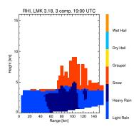
Figure 4.11: Hydrometeor classification derived from the synthetic polarimetric quantities for the SynPolRad simulations only considering rain.
