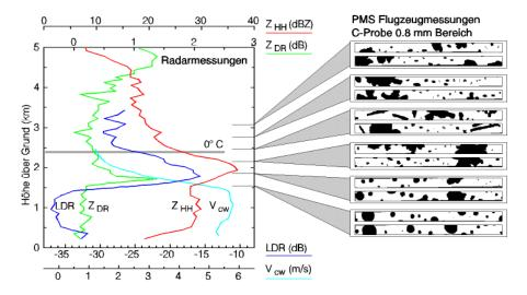
Figure 4.6: Vertical profiles of  $Z_{HH}$  [dBZ],  $L_{DR}$  [dB],  $Z_{DR}$  [dB], and terminal falling velocity  $V_{cw}$  [m s<sup>-1</sup>] measured by POLDIRAD together with particle images recorded by the PMS 2D cloud particle probe measurements (0.8 mm range) on board of the DLR Falcon aircraft (Hagen et al. (1993)).
