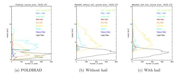
Figure 6.21: Vertical distribution of hydrometeors for an observed and simulated volume scan for the French research model MesoNH in the model versions without and with hail at 19:00 UTC.
