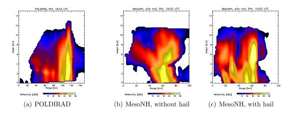
Figure 6.22: Observed (19:23 UTC) and simulated RHI of reflectivity [dBZ] for the MesoNH at 19:00 UTC.
