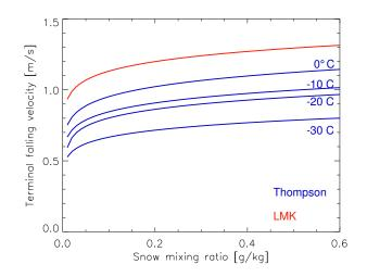
Figure 5.11: Comparison of terminal falling velocities of snow  $[m s^{-1}]$  as a function of snow mixing ratio  $[g kg^{-1}]$  for the LMK 3 component scheme and the Thompson scheme for selected temperatures [° C].
