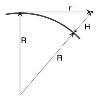
Figure 3.5: Geometry of the radar beam assuming linear propagation.  $\mathbf{H}$  is the height above ground,  $\mathbf{r}$  the range of the radar beam in the atmosphere, and  $\mathbf{R}$  is the earth radius.
