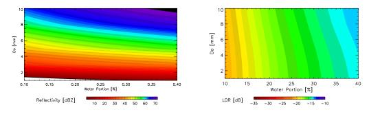
Figure 4.8: Reflectivity [dBZ] and  $L_{DR}$  [dB] as a function of the mean diameter [mm] and the water portion [%].
