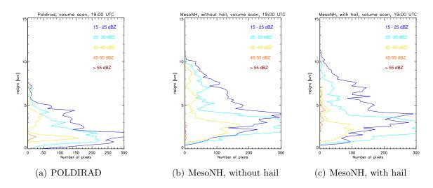
Figure 6.20: Vertical distribution of classes of reflectivity [dBZ] for an observed and simulated volume scan for the French research model MesoNH in the model versions without and with hail at 19:00 UTC.
