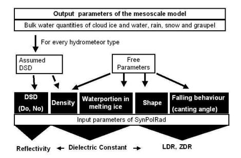
Figure 4.1: Conceptual view of the link between the NWP model and the polarimetric radar forward operator SynPolRad showing the input parameters defined by the model as well as the free parameters.
