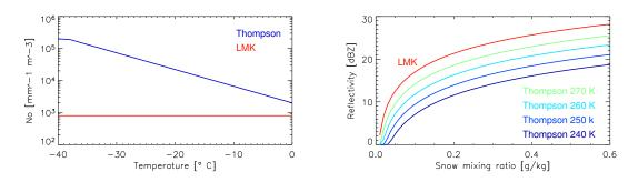
Figure 5.7: Left: The snow intercept parameter  $N_o \, [\text{mm}^{-1} \, \text{m}^{-3}]$  as a function of temperature [° C] for the LMK and the Thompson scheme. Right: Reflectivity [dBZ] as a function of snow mixing ratio  $[\text{gkg}^{-1}]$  and temperature [K] derived for the LMK 3 component and the Thompson scheme.
