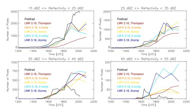
Figure 6.6: Time series of histograms derived from observed and simulated 1° PPI scans for different classes of reflectivity [dBZ]. The POLDIRAD observations are given in black while the model runs are plotted in colour.
