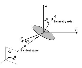
Figure 3.3: Scattering geometry where  $\vec{N}$  is the symmetry axis of the scatterer.  $\Psi$  is the conventional radar elevation angle, V and H are the linear polarization base vectors, and  $\vartheta$  is the canting angle of the scatterer. The incident wave is assumed to propagate along the -X direction (see also Vivekanandan (1986)).
