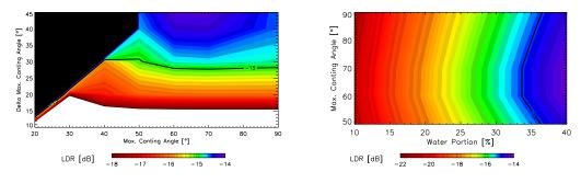
Figure 4.7: Left:  $L_{DR}$  [dB] as a function of the maximum canting angle  $\vartheta$  and its standard deviation  $\Delta \vartheta$  for a fixed water portion of 40%. Right:  $L_{DR}$  [dB] as a function of maximum canting angle  $\vartheta$  and the water portion [%] in melting ice. The chosen threshold of a  $L_{DR}$  value of -15 dB is given as a black graph.
