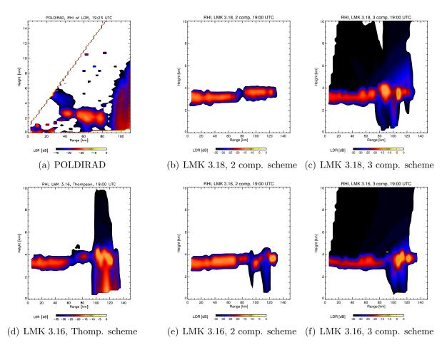
Figure 6.15: Observed (19:23 UTC) and simulated RHI of  $L_{DR}$  [dB] for different model versions of the LMK at 19:00 UTC.
