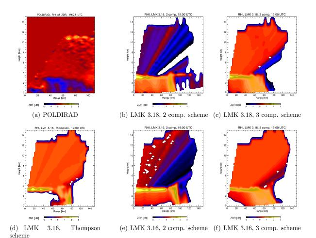
Figure 6.14: Observed (19:23 UTC) and simulated RHI of  $Z_{DR}$  [dB] for different model versions of the LMK at 19:00 UTC.
