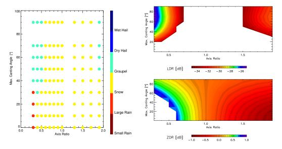
Figure 4.5: Left: Classification of hydrometeors as a function of axis ratio and maximum canting angle for a fixed density of  $\rho = 0.2 \text{ g cm}^{-3}$ . Right: Variability of  $L_{DR}$  and  $Z_{DR}$  as a function of axis ratio and maximum canting angle. Shown are only values within the thresholds for graupel from the hydrometeor classification scheme.
