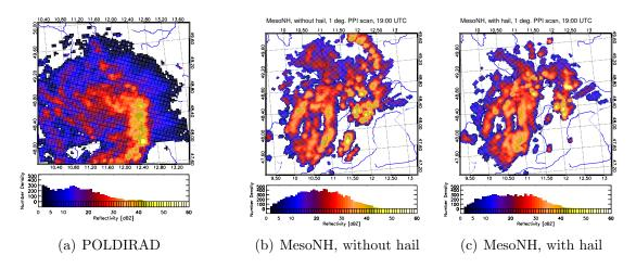
Figure 6.19: Observed and simulated 1° PPI scans of reflectivity [dBZ] for the French research model MesoNH in the model versions without and with hail at 19:00 UTC.
