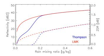
**Figure 5.4:** Reflectivity [dBZ] (solid line) and  $Z_{DR}$  [dB] (dashed line) for the LMK and the Thompson schemes as a function of rain mixing ratio [g kg<sup>-1</sup>].
