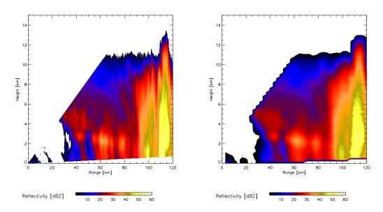
Figure 3.6: Comparison of POLDIRAD RHI scan in its original resolution (left) and interpolated on a vertical resolution of 200 m (right).
