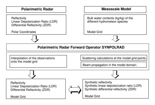
Figure 3.2: Flow chart of the processing of model and radar data by SynPolRad.
