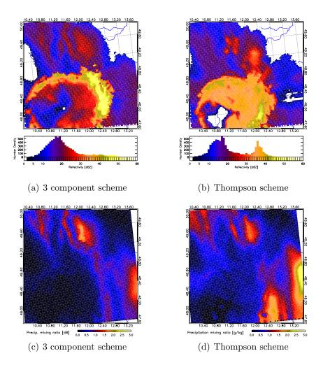
**Figure 5.5:** Synthetic 1° PPI scan of reflectivity [dBZ] (upper row) for the LMK 3.17 considering the 3 component and the Thompson scheme and the precipitating water mixing ratio [g kg<sup>-1</sup>] along the path of the radar beam for the two model configurations at 8:00 UTC.
