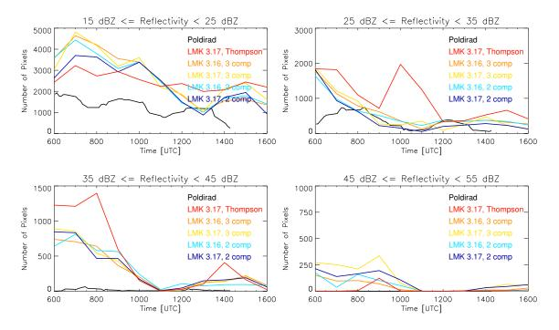
Figure 5.2: Time series of histograms of observed and simulated 1° PPI scans in different classes of reflectivity [dBZ] for July 5th, 2005.
