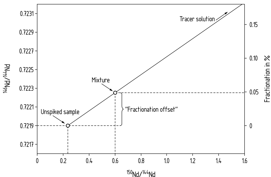
Figure 18: The ^{146}\text{Nd}/^{144}\text{Nd} ratio of a sample–spike mixture as a function of its ^{150}\text{Nd}/^{144}\text{Nd} ratio (calculated for the Munich ^{150}\text{Nd} tracer solution). The true ^{146}\text{Nd}/^{144}\text{Nd} ratio of the mixture is unknown at the time of the mass spectrometric analysis. Instead, the natural ^{146}\text{Nd}/^{144}\text{Nd} ratio of 0.7219 is used for correction, resulting in an incorrect normalization. This incorrect normalization—which may be named ‘fractionation offset’—has to be accounted for in a second-order correction. It can be seen that the fractionation offset is small for the chosen ^{150}\text{Nd}/^{144}\text{Nd} ratio of 0.6, keeping the extra uncertainty introduced by the second-order mass fractionation correction small. See text for discussion.
