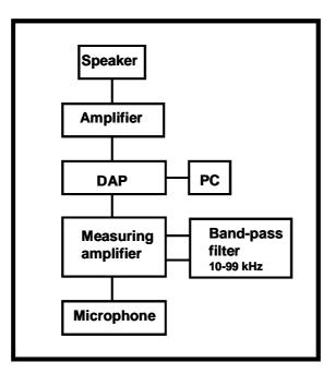
Figure 25: Block diagram for the impulse response playback set-up
