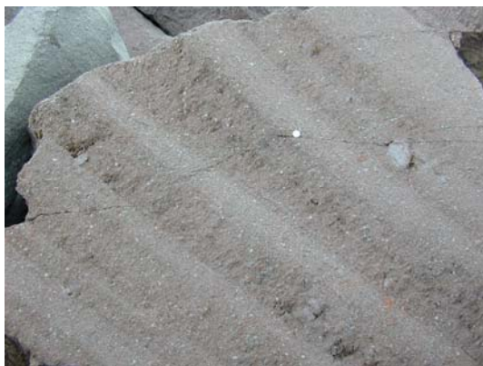
Fig 10 (left): The porosity was often arranged in layers of several centimetres to a few decimetres (width of picture is 1 m).
