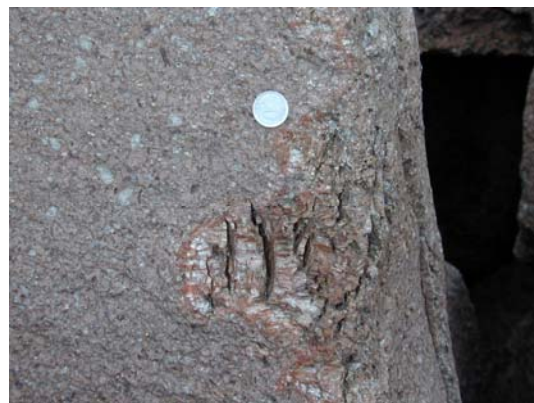
Fig 10 (left): The porosity was often arranged in layers of several centimetres to a few decimetres (width of picture is 1 m).
