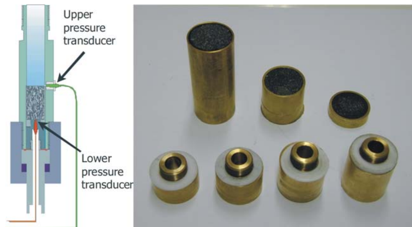
Figure 5.4: Setup to investigate the pressure profile within a sample. It is very similar to the setup used for the fragmentation speed analyzes. The sample is stepwise sliced down from 60 mm to 4.6 mm. The shortened sample was compensated with distance holder placed below the lower transducer.
