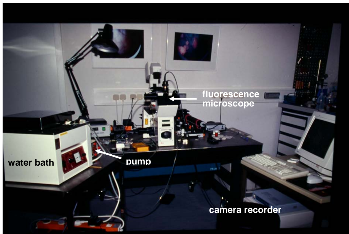
Figure 11: Experimental set-up for recording of fluorescence of co-cultures. The temperature in the co-culture was controlled by pumping water from the 37°C bath (left, foreground) through the incubation chamber mounted on the confocal microscope. The recorded fluorescence was directly processed and displayed on the computer screen.
