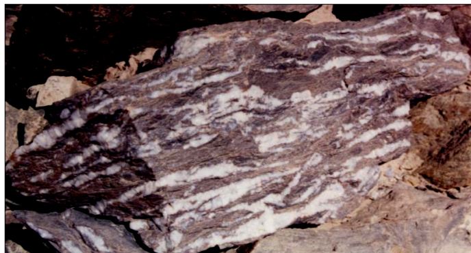
Fig. (4.9): Densely veined wallrocks from zones adjacent to the main gold-bearing veins in the Um El Tuyor mine. The quartz veinlets are disposed along foliation planes (wide of view is ~20 cm).
