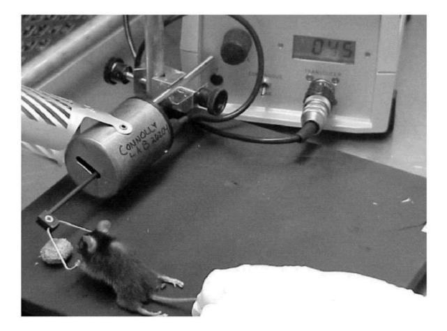
**Fig. 2-2 Grip strength measurement.** After it has gripped the trapeze the mouse is gently pulled backwards until it releases its grip. Grip strength is measured by a force transducer and recorded by a computer. (after Connolly et al., 2001)
