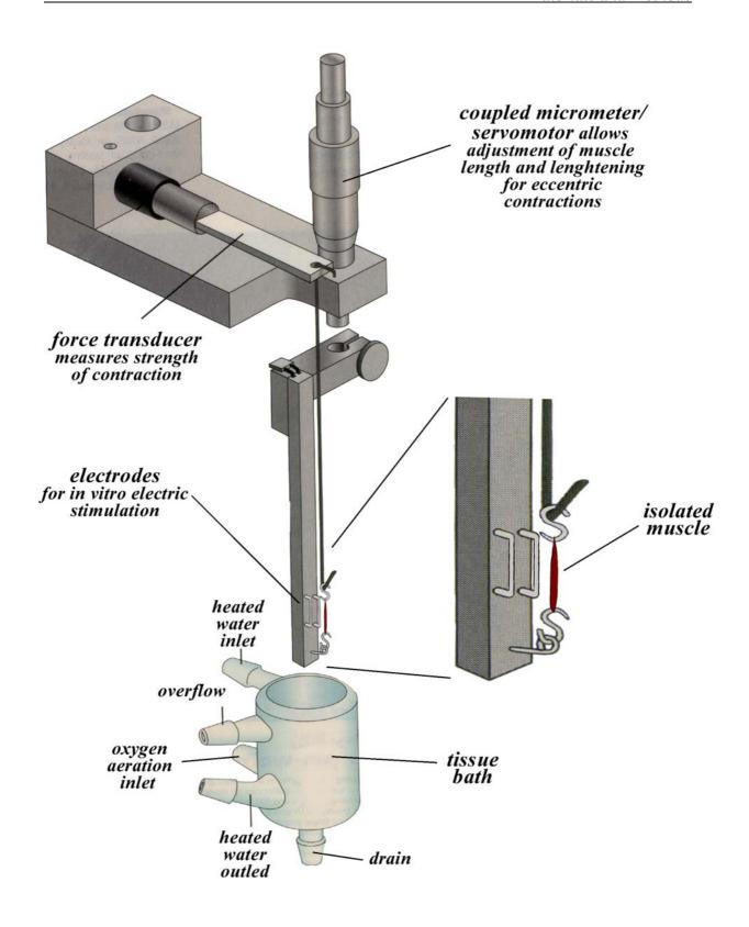
**Fig. 2-1 Equipment for force measurement of isolated muscle.** (adapted from World Precision Instruments, Berlin, Germany 1999)
