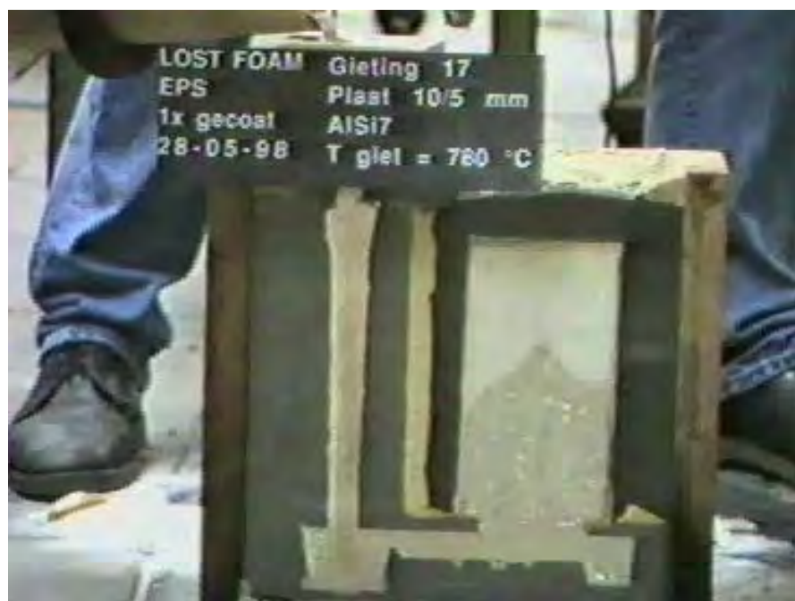
Figure 2.39: Single frame of a video used to record the filling of a Lost Foam mould through a transparent window ( courtesy of Lovink B.V., The Netherlands )
