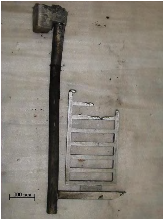
Figure 4.25: Bottom-gated frame casting ( made as part of the real time X-ray mould filling analysis. Reference Figure 4.22 and 4.23 )
