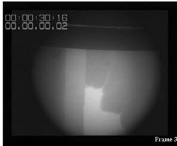
Figure 5. Real-time X-ray image of the filling of a Lost Foam plate pattern with a top-gated running system.
