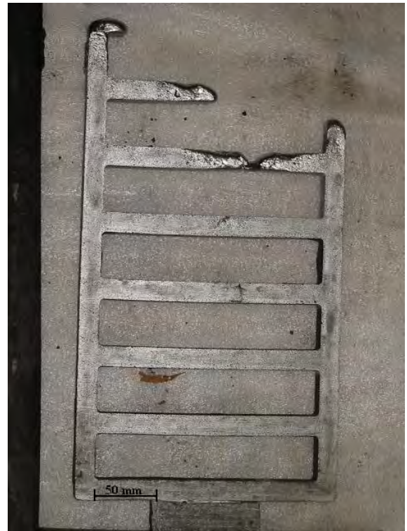
Figure 4.25: Bottom-gated frame casting ( made as part of the real time X-ray mould filling analysis. Reference Figure 4.22 and 4.23 )
