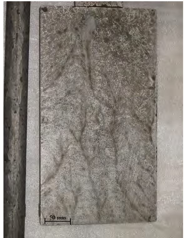
Figure 4.14: Top-gated plate casting ( made as part of the real time X-ray mould filling analysis. Reference Figures 4.10 and 4.11 )
