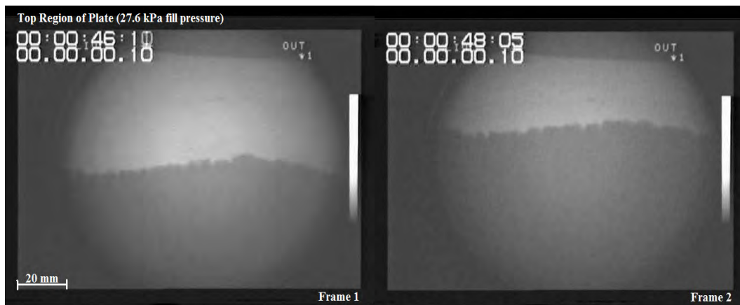
Fig 5 Irregular Metal Front in the Upper Region of a Plate (Fill Pressure = 27.6 kPa)
