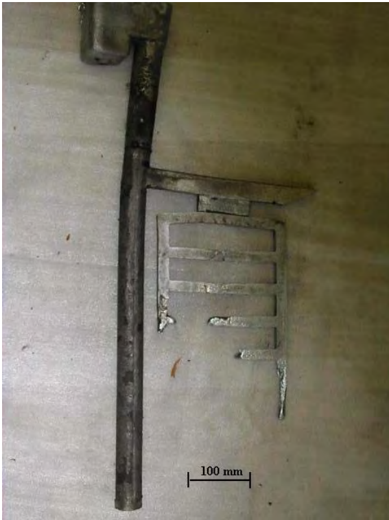
Figure 4.24: Top-gated frame casting ( made as part of the real time X-ray mould filling analysis. Reference Figure 4.20 and 4.21 )
