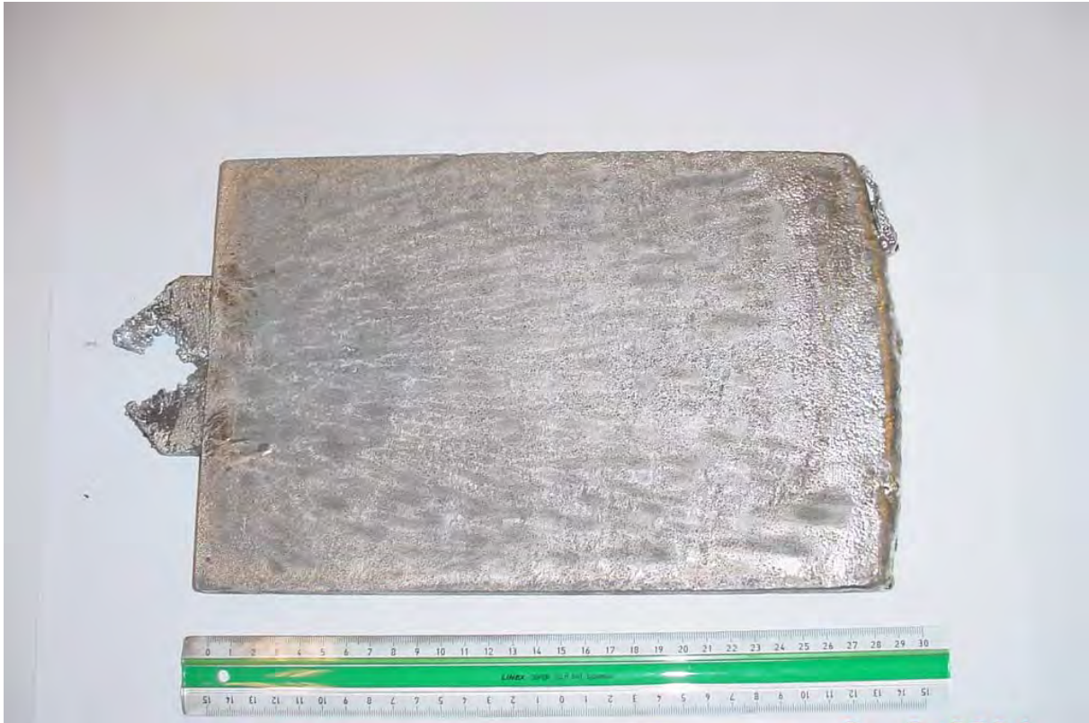
Figure 4.46: Counter-gravity filled plate casting made at a vessel pressure of 24.1 kPa. (made as part of the real time X-ray mould filling analysis. Reference Figure 4.44 and 4.45).
