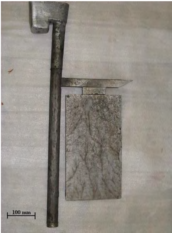
Figure 4.14: Top-gated plate casting ( made as part of the real time X-ray mould filling analysis. Reference Figures 4.10 and 4.11 )
