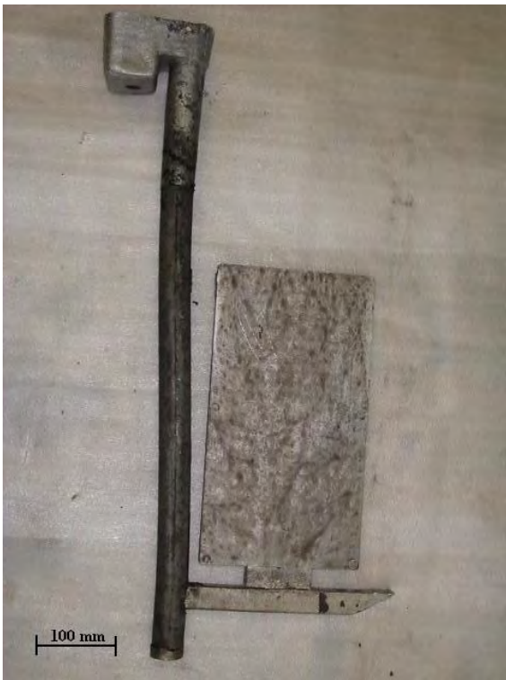
Figure 4.15: Bottom-gated plate casting ( made as part of the real time X-ray mould filling analysis. Reference Figures 4.12 and 4.13 )
