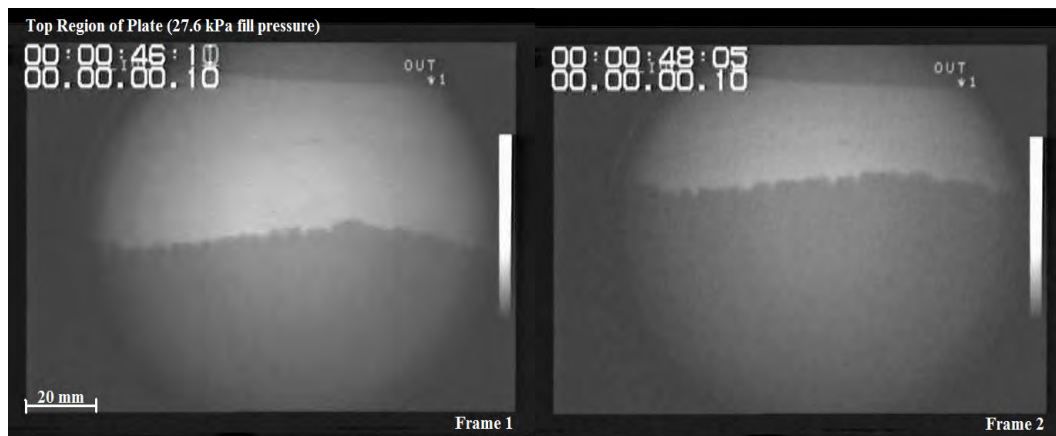
Figure 8. Real-time X-ray image of the filling of a Lost Foam plate pattern at a velocity of about 13 \text{ mm.s}^{-1} .
