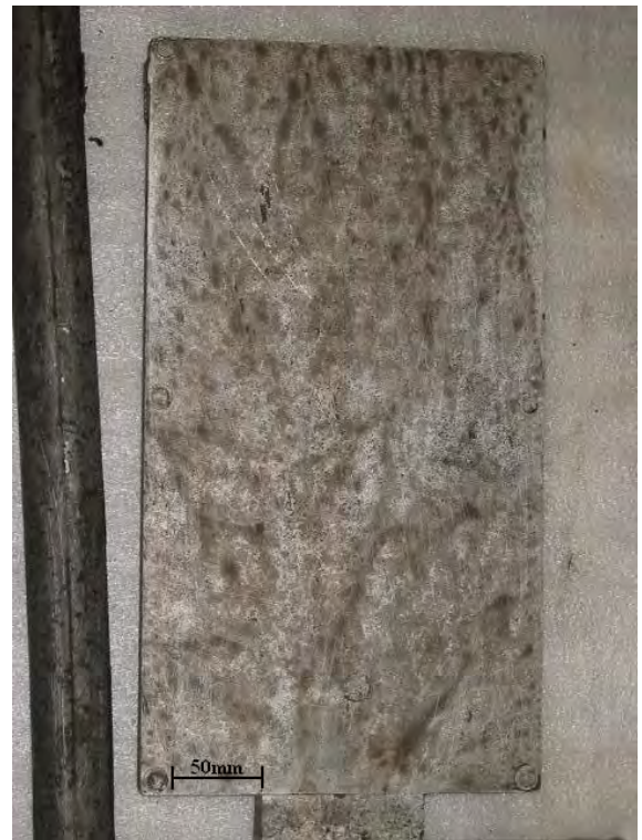
Figure 4.15: Bottom-gated plate casting ( made as part of the real time X-ray mould filling analysis. Reference Figures 4.12 and 4.13 )
