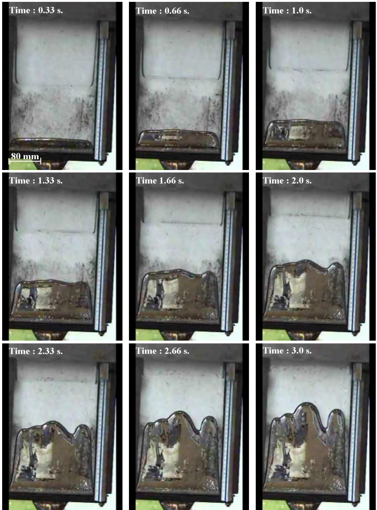
Figure 4.66: Displacement of glucose syrup with a dynamic viscosity of 35 Pa.s and confined between glass plates by liquid mercury travelling at approximately 70 \text{ mm.s}^{-1} .
