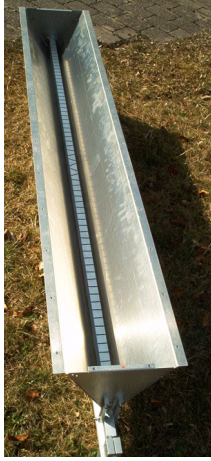
Figure 3.2: Photograph of a bistatic antenna consisting of a slotted waveguide in the center surrounded by a triangular reflector (front panel removed).
