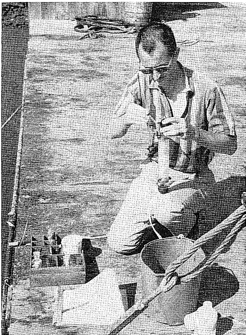
Fig. 8. Mr. J. R. Grady using the Emery oxygen bottle during a 24 hourly-series of hydrographic measurements at the cannery pier.
