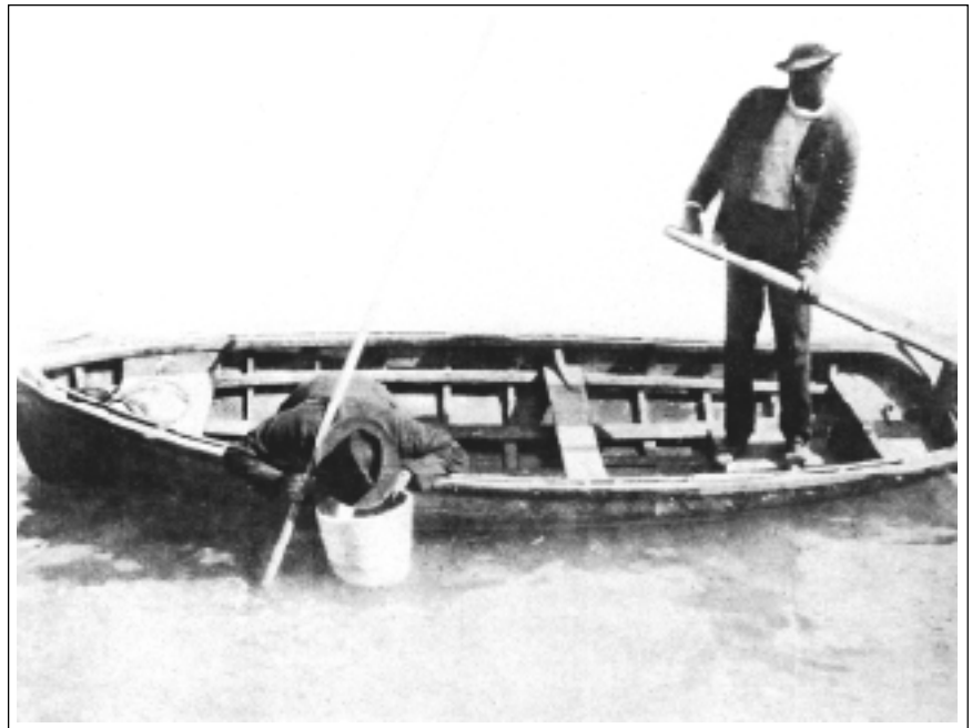
Figure 6.—Florida sponge skiff with sculler at the oar and the hooker looking for sponges through the glass box (Cobb, 1904).
