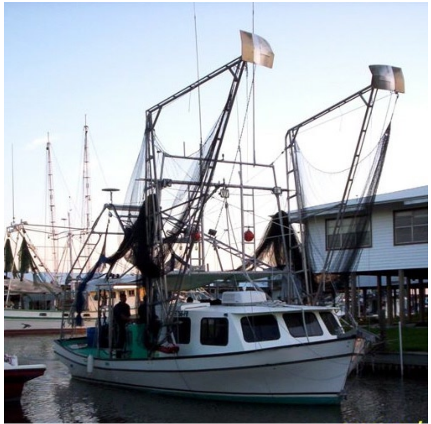
Figure 1.—A skimmer trawl vessel showing the paired-frame net design.
