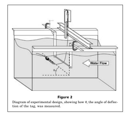
scale by loops tied at either end. One loop was threaded through the release pin in order to lasso the tag. The other loop was then attached to the clip on the spring scale and the tag was passed under the Delrin rod so that it floated to the other side (Fig. 2). The depth of the Delrin rod and the length of the monofilament were selected so that the tag was completely immersed in the water throughout the experiment and so that it floated within
