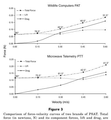
force (in newtons, N) and its component forces, lift and drag, are plotted against flume velocity (m/s). The angle of deflection of the PSAT as measured upward from horizontal is indicated above each set of points
