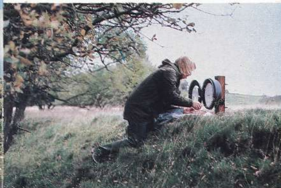
9.4 Changing a thermograph chart on a Teesdale stream.
