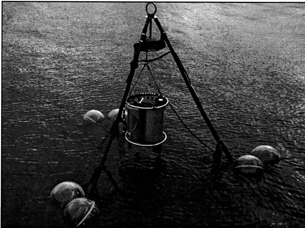
Figure 2. Tetrahedron surface floatation used in MOS radiometer profiling.
