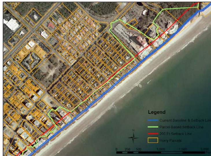
Figure 3: Current baseline and setback line, conceptual parcel-based setback line, and conceptual uniform 200-ft setback line for Myrtle Beach, SC.
