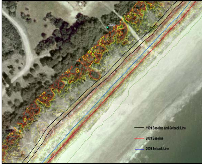
Figure 1: 1999 and 2009 (revised) baseline and setback line positions for a portion of Huntington Beach State Park, SC. A new dune line has formed seaward of the previous dune line following renourishment projects. The revised baseline and setback line moved about 85 feet seaward to the new primary dune.
