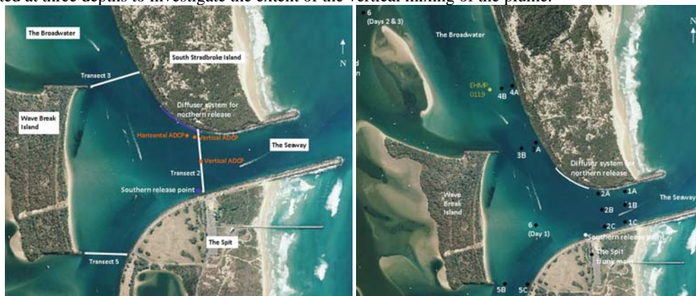
Figure 1. Location of ADCPs (Source: Gold Coast City Council). Figure 2. Water quality monitoring sample points (Source: Gold Coast City Council).
