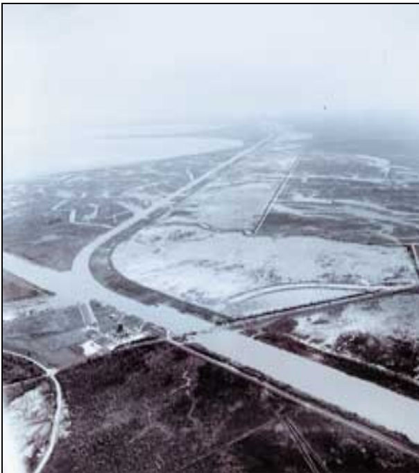
Figure 8: Photos of the Mississippi River Gulf Outlet taken in 1960 (left) and 1989 (right), looking southeast at the junction between the MRGO and the Intracoastal Waterway. Notice the extent to which the MRGO has widened with its southward flow from the ICWW, and the decay of the adjacent wetlands in the left-center of the photos. Photos courtesy of Louisiana Sportsman Magazine .
