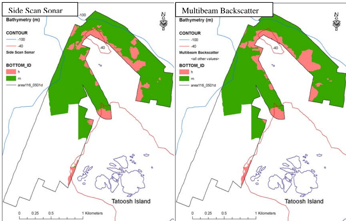
Figure 10. Footprint of survey block 116_0501d (black outline) showing overlapping areas mapped with both types of sonar (shaded polygons). Results of texture classification are based on side scan sonar imagery (left) and multibeam backscatter (right). Note the overall similar results with only one small area of hard bottom recognizable in the side scan imagery being lost in the backscatter classification. green = mixed (m), and red = hard (h).
