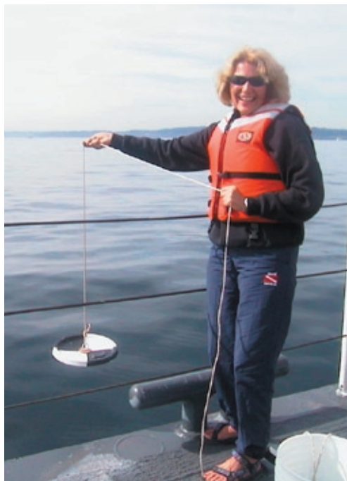
Figure 5. Pam Polmateer prepares to take a secchi disk depth reading in the Puget Sound near Seattle, Washington. Photo courtesy of Felicity Burrows, NOAA National Centers for Coastal and Ocean Science.
