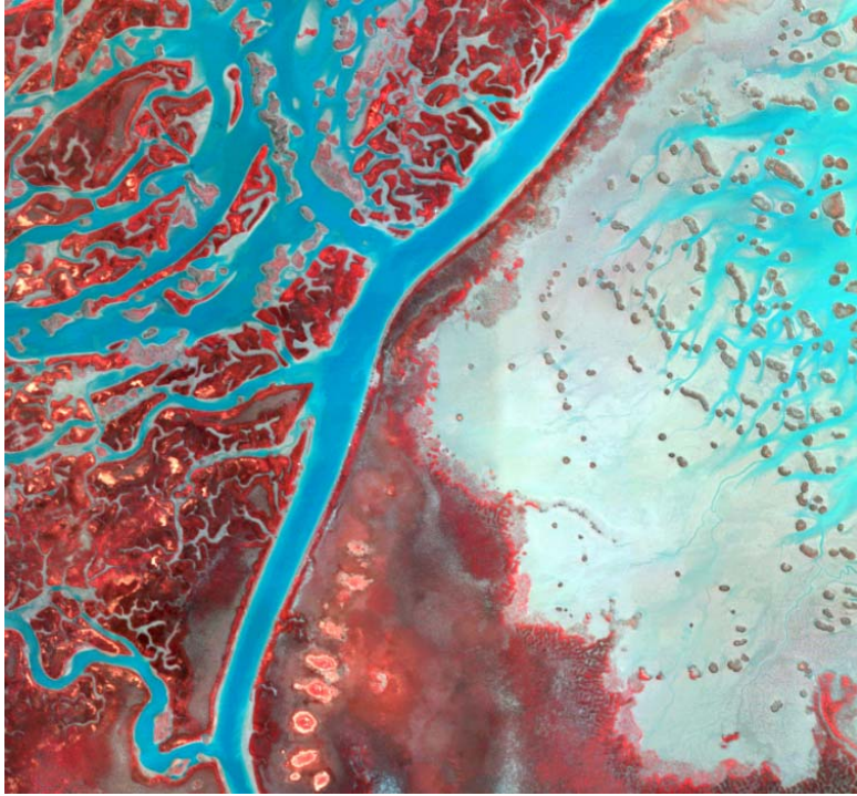
Figure 5. Near infrared composite GeoScanner image of the Hamlin Creek area. Pixel size is 0.25 meters. This imagery has four discrete spectral bands that support automated image processing algorithms. The image on the left is a mosaic of many individual image frames.
