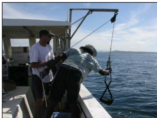
Sampling for sediment with the Van Veen grab.
